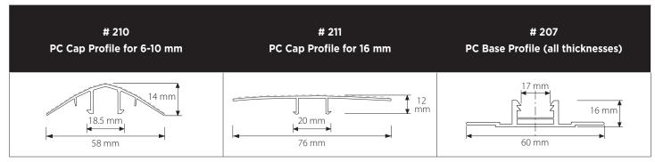
**Easy Clip (ECP) connection profiles** are for use with sheets having a thickness from 6 to 10 mm and can be used in a wide variety of DIY, simple architectural and agricultural applications.
