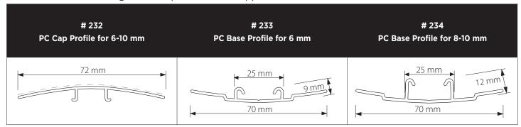
**GCP (Gasket Clip Profiles) connection profiles with integrated gaskets** are intended for use with sheets having a thickness from 6 to 10mm sheets and are designed for greater water sealing capability. This system can be used in a wide variety of DIY, simple glazing and agricultural applications. The profiles have a "snap-and-click" design for connecting of base and cap profiles.
